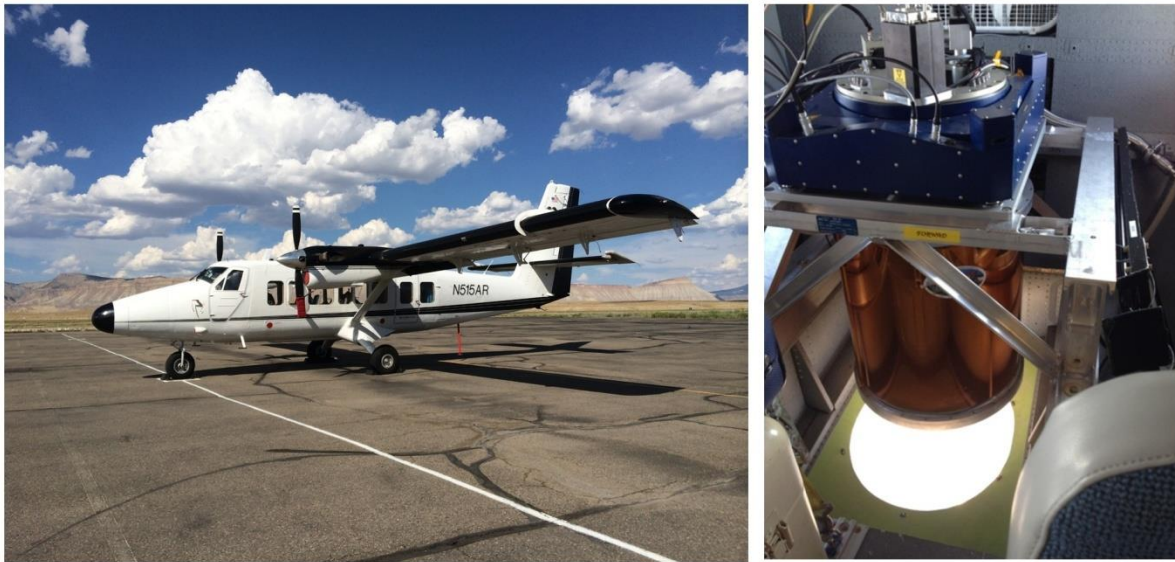
Figure 3. HyTES installation in Twin Otter aircraft.
